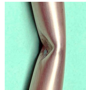
Figure 7: Bend at the half-flattened spot.
