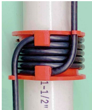
Figure 10: 1:1 mini-8 coax choke balun on 3D printed bobbin
